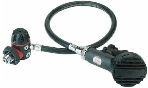
The balanced diaphragm means that the effort to open and close the first stage valve is unaffected by changes in tank pressure or depth. The balanced design allows for a larger first stage orifice, which improves regulator performance. The design of the diaphragm does not allow water to enter the first stage, which means no salt, sand, or other contaminants will build up on the internal surfaces of the regulator.
