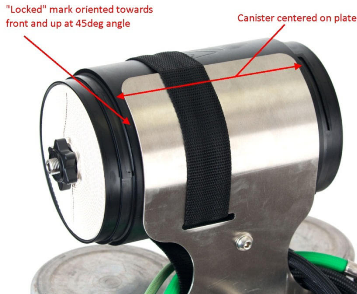
Figure 10 - Scrubber Canister Installation
