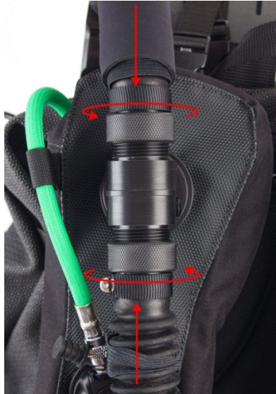
Figure 27 - Installing Loop Hoses
