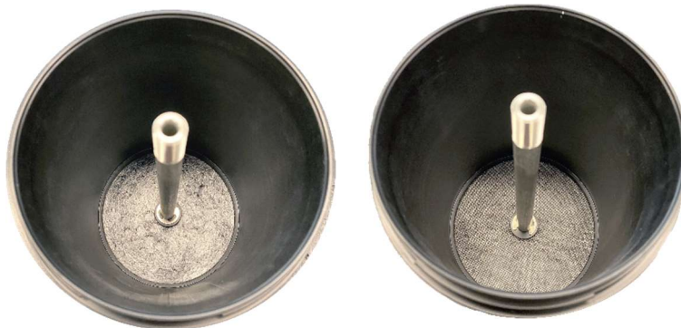
Figure 4 – Filter and Screen Installed in Scrubber Canister
