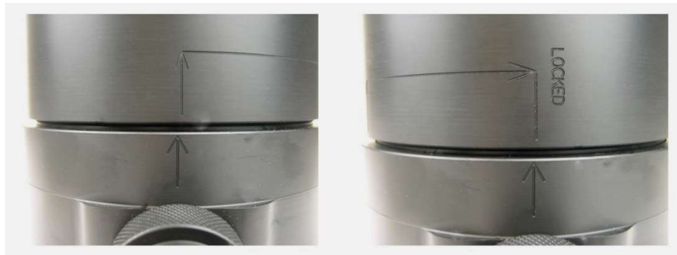
Figure 11 – Installing Electronics Head
